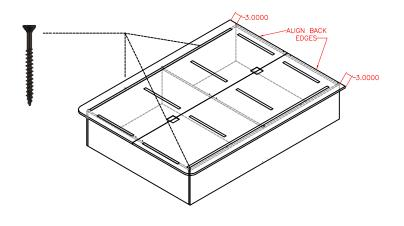
STEP 8: INSTALL THE 3X3 FLAT BRACKETS INTO THE BRACKET POCKETS ON THE TOP PANELS.
