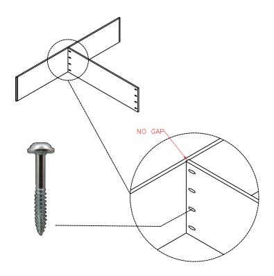
STEP 4: ATTACH CENTER SUPPORT PANEL TO SECOND SIDE PANEL.
